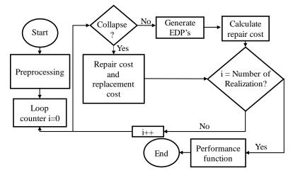
Figure 4. The flowchart of the performance-based loss assessment procedure in the current version of FEMA P-58.
