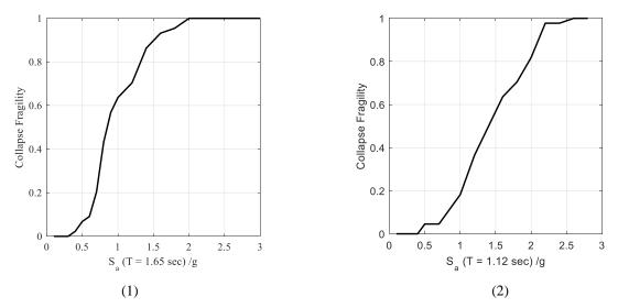
Figure 2. Building Collapse Fragility: (1) steel moment frame (2) reinforced concrete moment frame.
