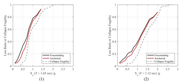
*Figure 5. Content vulnerability function: (1) steel moment frame (2) reinforced concrete moment frame. Dashed lines indicate the building's overall collapse fragility curves.*
