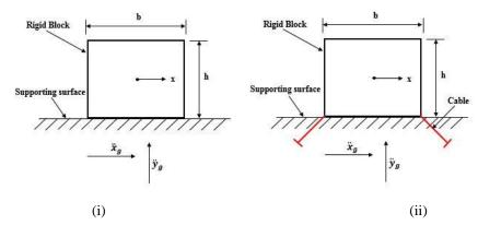
Figure 1. Rigid block models: (i) Free Standing (ii) Anchored
